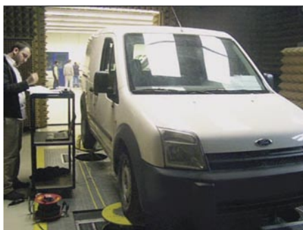
▲ The Ford Transit Connect with semi-active suspension controller is being tested on a four-poster.
